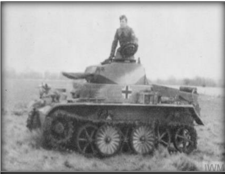
Germany's first modern tank. With a top speed of 79km/h Panzer I C series.
